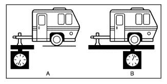
If you are using a weight-carrying hitch or a weight-distributing hitch, the trailer tongue (A) should weigh 10 to 15 percent of the total loaded trailer weight (B).
